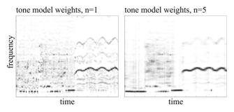
Figure 2: Effect of window size n on the EM algorithm for predominant pitch estimation
