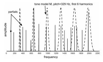
Figure 1: Applying a tone model on a set of partials
