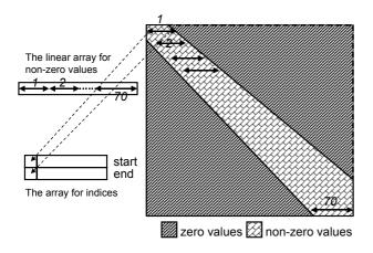
Figure 4: The reduction method "Storage in two arrays."
