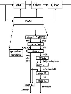
Figure 1: *The spreading function of psychoacoustic model in an AAC encoder.*
