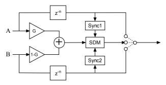
Figure 6: Smooth switching between bitstreams using synchronisation.
