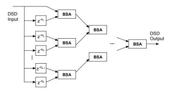
Figure 3: Implementation of a basic flanger or chorus using the bitstream adder (BSA) of Figure 2.
