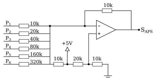
Figure 6: Sawtooth waveform generation in the ARP Pro Soloist. The input square wave signals  $P_1, \dots, P_6$  are generated by a top octave divider.  $P_1$  is the lowest generated octave, corresponding to the note fundamental.
