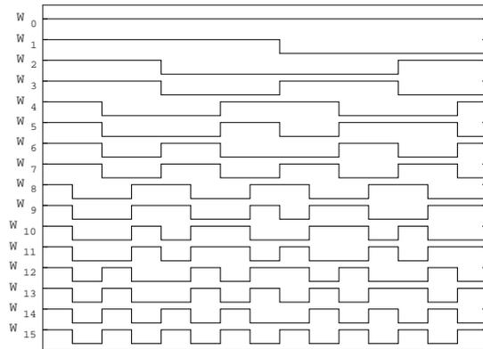
Figure 1: Walsh matrix of order  $M = 16$ , plotted row-wise. The signals constitute orthogonal bases that are employed in the Walsh transform. The first line corresponds to Walsh function of order 0 (DC), or  $W_0$ , while the last has index  $M - 1$ .
