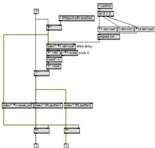
Figure 2: Spectral delay abstraction.
