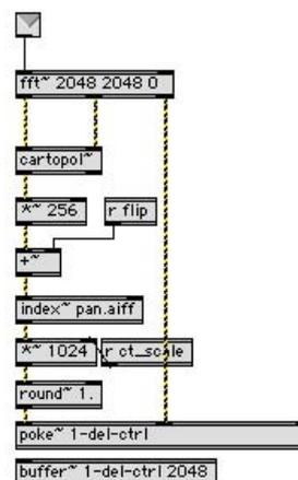
Figure 4: Signal control of delay times.
