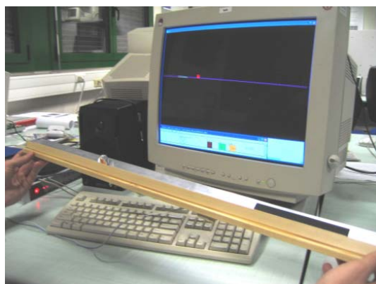
Figure 1: The Ballancer with the graphical display spanning the whole 21" monitor (display factor 12). The photo was taken during use of the device in a game application, thus the lighter target area on the screen is not in the same fixed position as during the performance task described here (slightly right from the middle, according the black mark on the mechanical track). Also, the real glass marble on the track only serves demonstration purposes in the photo.
