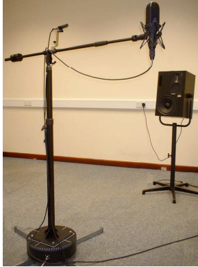
Figure 1: Measurement microphones mounted on a turntable and S30D sound source transducer.
