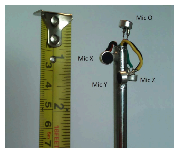
Figure 1: Configuration of the miniature XYZO array. The top microphone has an omnidirectional response and the bottom three microphones have gradient responses. Each sensor is 6mm (Diameter) \times 2.7mm (Height)
