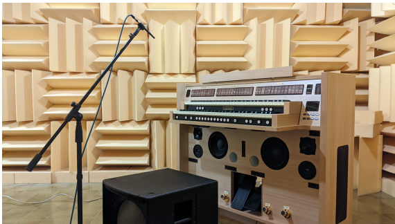
Figure 4: Picture of the organ under test. The loudspeakers IRs are measured to assess the validity of the method.
