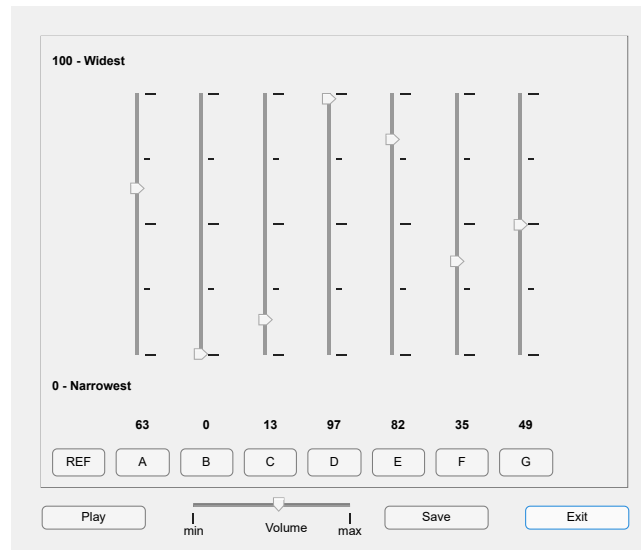
Figure 3: User interface for evaluating the perceptual correlation between ITLD and ASW using the MUSHRA framework.
