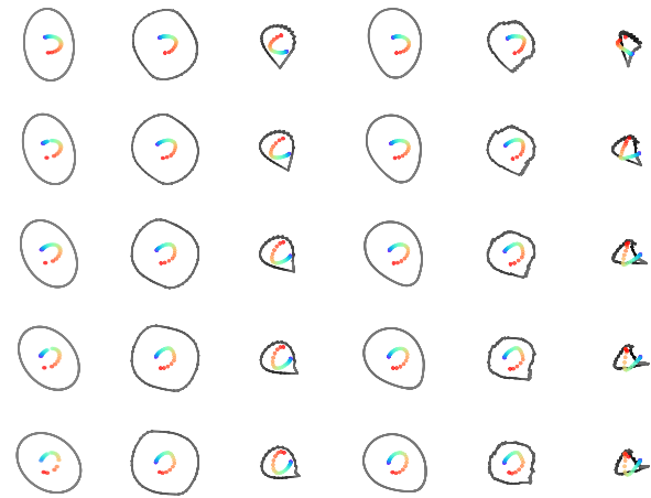
Figure 4: Visualization of the signals from Figure 1, now with N = 24 and d = (0, 1, 3, 6, 10, 15, \dots, 253, 276) . Now the shapes of the gray curves are very consistent in each column, and changes in frequency are recorded instead by the colorful spirals – the rows of A – which turn through a greater angle when the pitch is higher.
