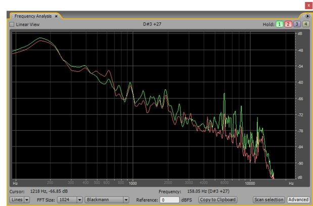
Figure 9: Frequency response of signal used for the masking procedure (red line) and its equalized version (green line).
