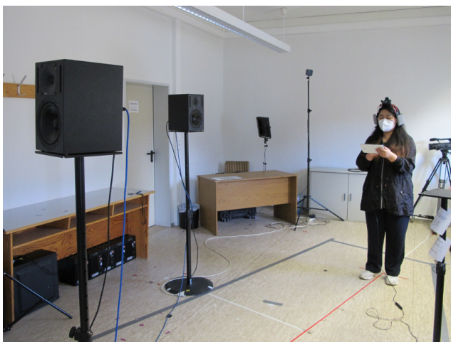
Figure 1: A participant exploring the real and virtual loudspeaker arrangement in the seminar room, illustrated in Fig.2. The participant wears a pair of AKG K1000 with the attached Generic Vive Tracker. The red line marks the explorable path. In this specific scenario, an arrangement where the frontal loudspeaker was turned around by 180° was chosen.
