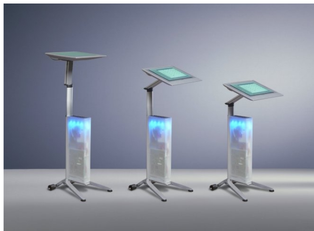
Figure 1: An example for a silent computer system in a hybrid environment: the ConnectTable ® is build upon computer components that emit no noise (Design: Fraunhofer IPSI, Wiege, Wilkhahn).
